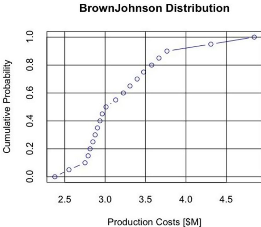
Figure 3-4. The cumulative probability distribution of the production costs using the piecewise linear BrownJohnson generator
